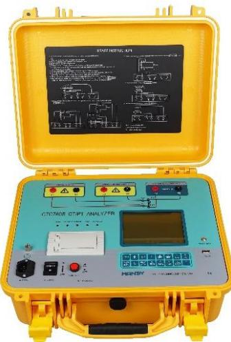
**CTC760E** Instrument transformer analyzer can carry out a series of standard tests quickly, such as determining the magnetization characteristic, saturation behavior (ALF/FS), transformation ratio and its accuracy, polarity, load, winding resistance, or remanence. Tests are performed in accordance with standards: IEC60044-1, IEC60044-6, IEC 61869, ANSI/IEEE C57.13.1.
