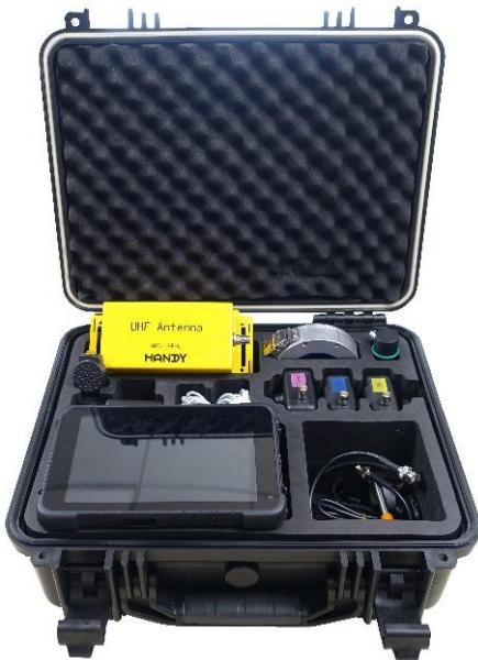
**HPD5000B** integrates multiple partial discharge detection functions and can use ultra-high frequency (UHF), high-frequency current (HFCT), transient earth voltage (TEV), and acoustic emission (AE) sensors for partial discharge detection of high-voltage equipment. It is suitable for live inspection of GIS, switchgear, cables, transformers, and other equipment.
